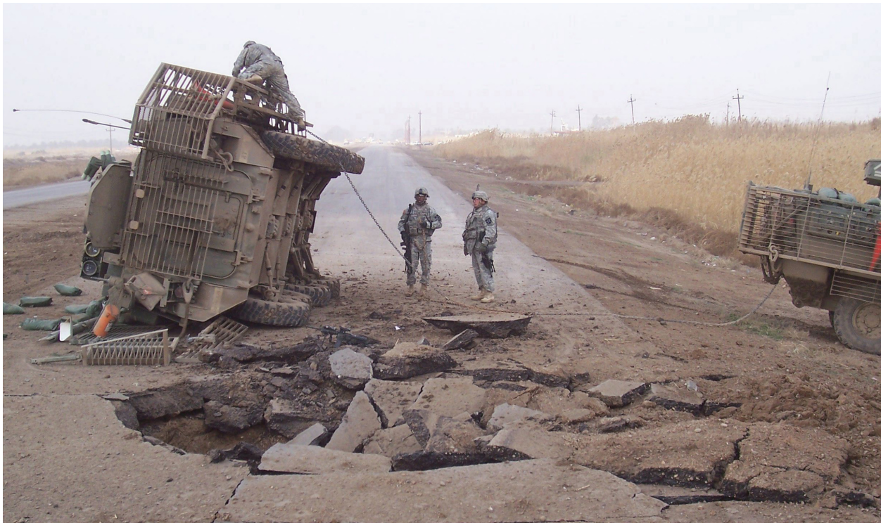
Figure 5: The Stryker vehicle "General Lee" lies on its side after surviving a buried IED blast in 2007. The vehicle was recovered and served several more missions until another bomb finally put it out of action. Photo by courtesy of the U.S. Army's 2nd Stryker Brigade.
