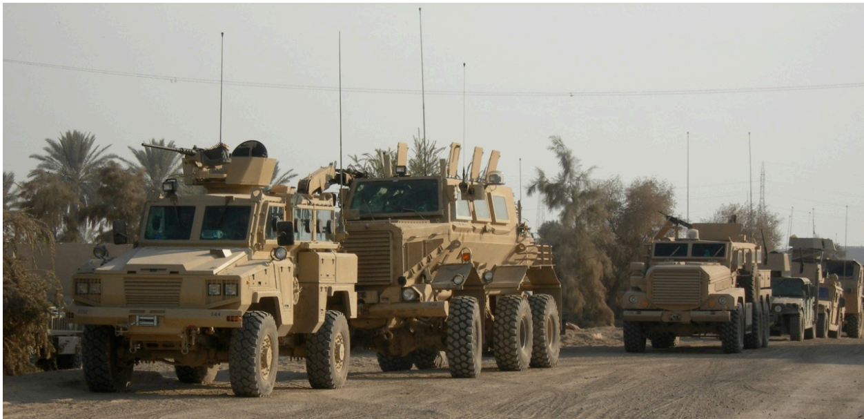
Figure 6: A column of MRAP vehicles in Iraq in 2005: a Cougar and a Buffalo from Force Protection Industries, followed by an RG31 from BAE Systems. Photograph courtesy of Colonel Eric Peterson, U.S. Marine Corps Reserve.
